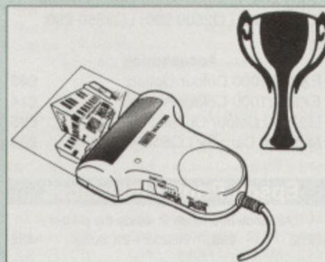
Watford Electronics are pleased to announce the launch of the first hand held scanner for the BBC Micro. HandScan is a compact unit which will allow photographs, diagrams, or any other documents to be digitised quickly and easily, to then be used in a desk top publishing package, art program, or even in your own Basic programs! These useful devices have been available for faster and more expensive micros for some time, but only now is Watford Electronics able to offer the BBC Micro computer.
