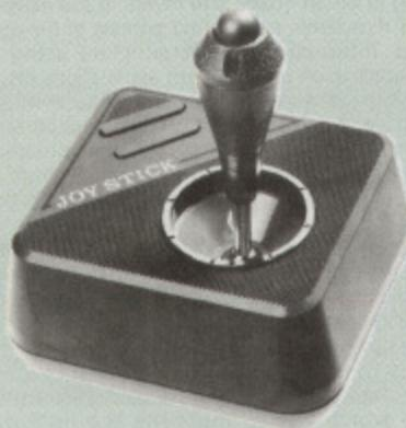
Watford Electronics' new Commander Joystick for the BBC B and Master 128K has a unique dual mode of operation giving selective free floating or self centring fully variable control in both X and Y axis directions. Commander is particularly good for flight simulation and drawing programs.
